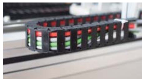
侧向架空安装拖链，一侧带支撑 The lying carrier, one side of the chain is supported
