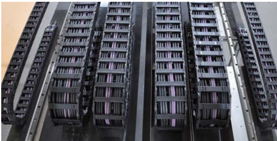
柔性电缆与拖链短行程架空耐久测试 Short-travel unsupported durability test for flexible cables and cable carriers
